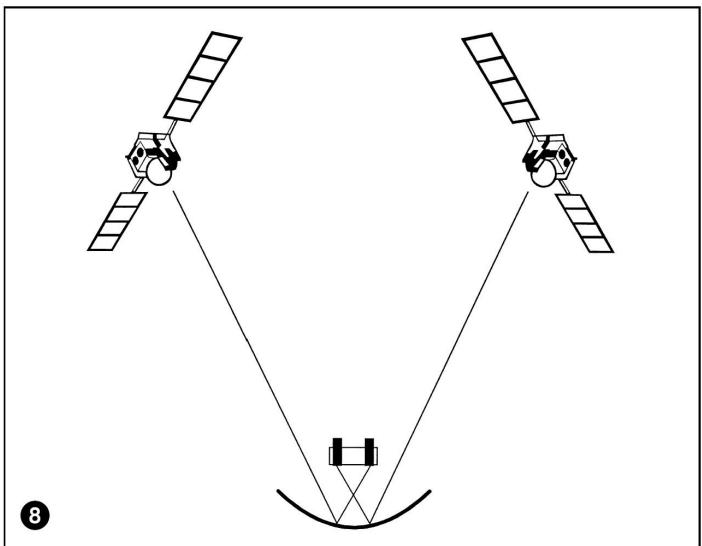
**Tip!** With multifeed applications the antenna should be aligned on the satellite with the weaker signal level.
