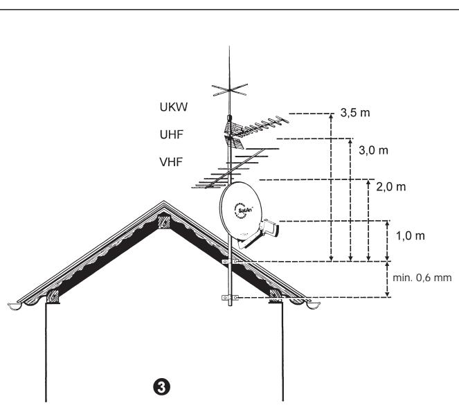
**Attention!** In case your antenna array wil be different, you must calculate the windload and bending moment acc. to DIN EN 50083-1 (or you ask a specialist to do it for you).
