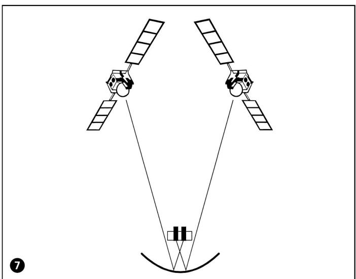
⑧ Example for mounting positions for multifeed reception from satellites 6° apart:
