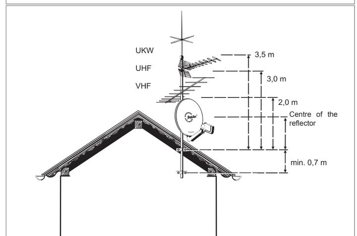
together with mast components from a specialist supplier (tube in steel grade St 52 with outside diameter 60 mm and wall thickness 2.5 mm at the mast clamping point – e.g. ZSH 59 from Kathrein).
